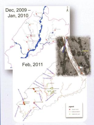
Embankment breach points are identified (table below) and mapped before the onset of flood season using CARTOSAT-1 stereo data and shared with Assam water resource department to enable them to take corrective measures.
